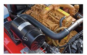
The standard engine is the high pressure common rail electronic-controlled engine which adopts high pressure multiple injections technology to ensure the strong power take-off, lower emission and better cold starting performance; saving the 10% of energy consumption.
