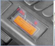
Newly-developed LCD instrument has more comprehensive functions and more stable performance and entirely displays the full truck running state, trouble diagnosis and other important information, which can make the operator more intuitively and conveniently have a better knowledge of truck state and make the maintenance conveniently.
